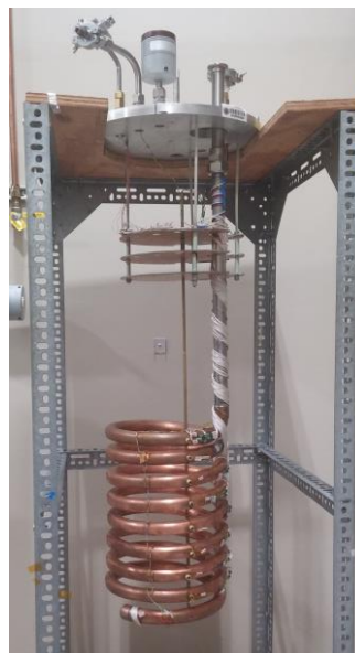
Figure 2. Internal assembly of helical tube system.
