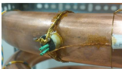
Figure 3. Stycast® epoxy encapsulated temperature sensor mounting on surface of helical tube system.
