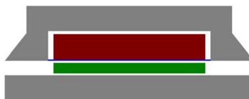
Figure 2. Linear motor with extended teeth.
