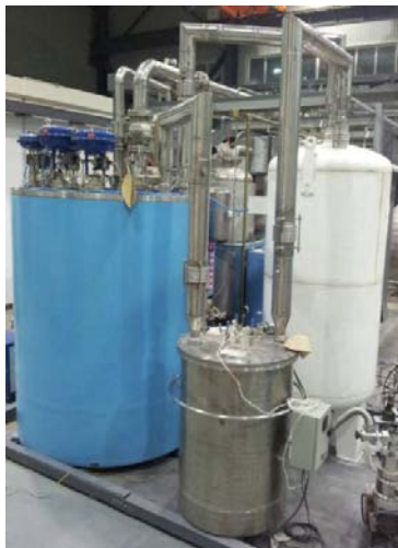
Figure 7. The 2kW/20K helium refrigerator in test site.
