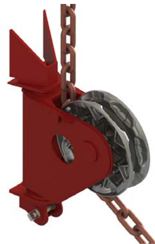
Figure 2. Sketch of mooring chain wheel at fairlead [11]
