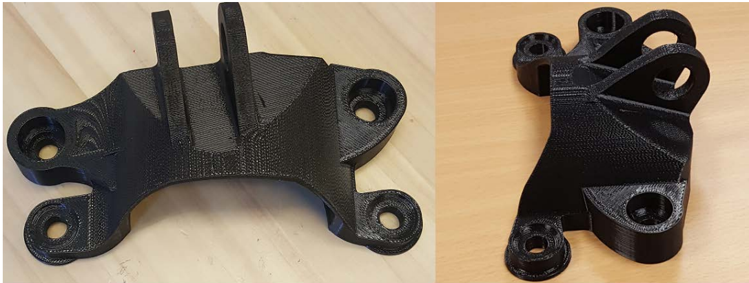
Figure 12. Additive manufactured final engine bracket design.
