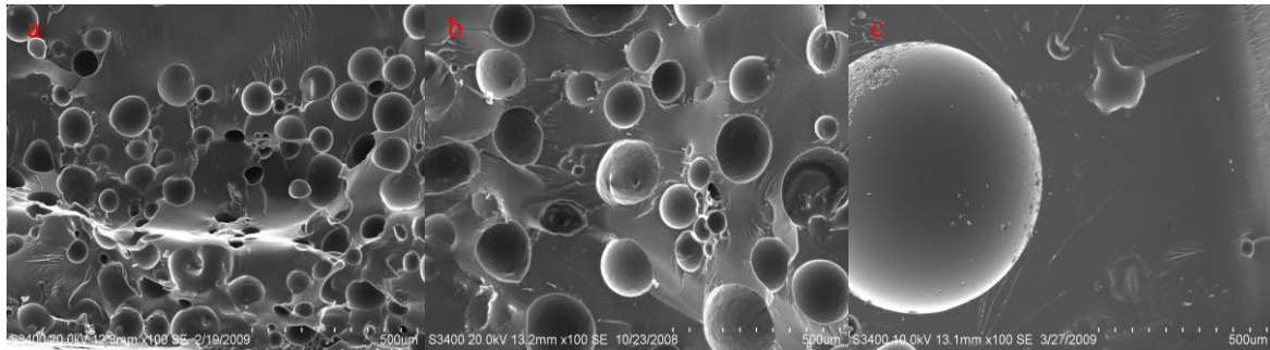
Figure 5. Effect of MUF microcapsules size on fracture morphology of epoxy composites (5wt% microcapsule content).
