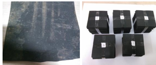
(1) Rubber cushion raw material (2) Test specimen after processing;
