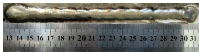
Figure 6. The welding seam with speed of 42cm/min
