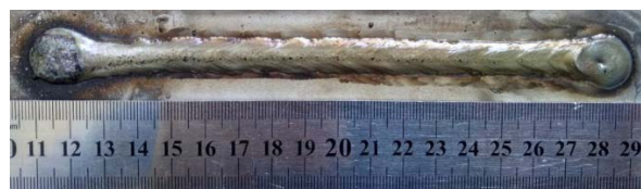
(a) The welding seam with speed of 36cm/min
