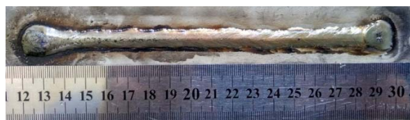
(b) The welding seam with speed of 48cm/min
