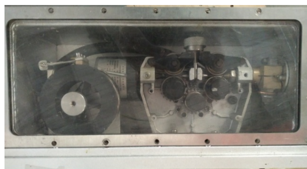
Figure 3. The diving wire feeder
