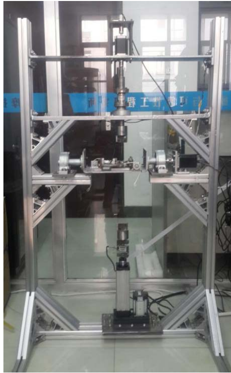
Fig 1. Schematic diagram of the mul-tiaxial fretting fatigue test rig of steel wire
