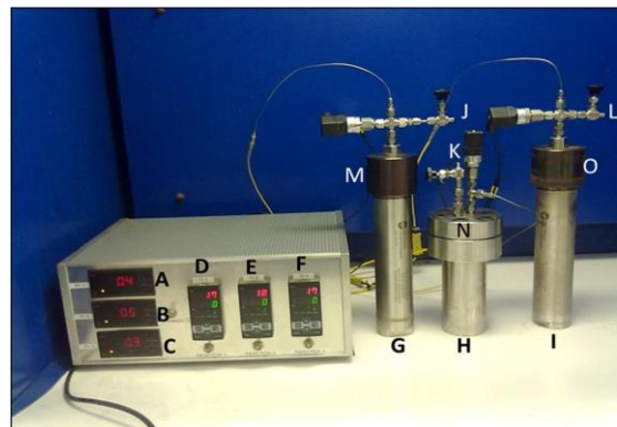
Figure 1. High pressure reactors (bolted and OC reactors).
