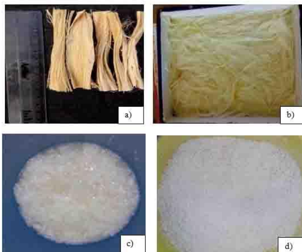
Figure 1. Various stages of microfiber extraction a) raw fiber b) bleached fiber c) oxalic treated fiber d) dried cellulose microfiber.
