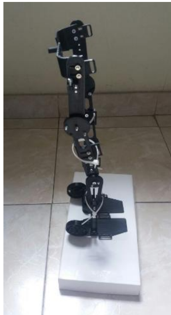
Figure 1. Exoskeleton controlled by movement intention.
