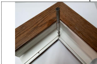
Figure 1. The inner countersink slot cleaning
