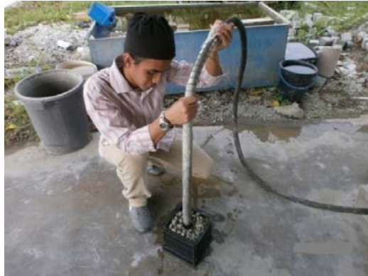
Figure 2. Vibration using poker vibrator
