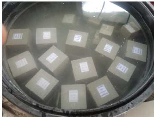
Figure 3. Concrete cubes subjected to water curing
