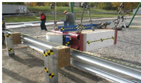
Figure 2. Impact test conducted by Virginia Technology [7].
