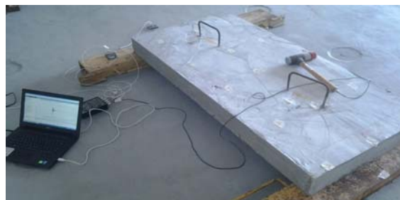
Figure 4. Test set-up for hammer-impact test.
