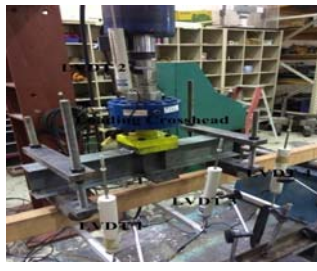
Figure 4. Arrangement of LVDT and Loading Crosshead
