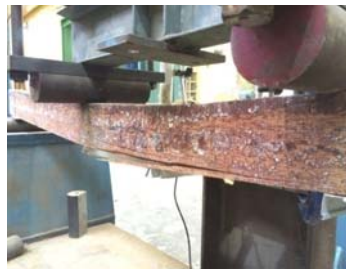
Figure 7. Mode of failure for Keruing
