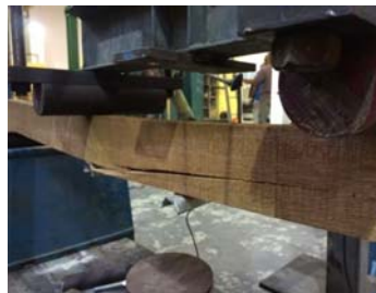
Figure 9. Mode of failure for Light Red Meranti
