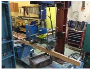
Figure 3. Timber Beam for Bending Test Set up
