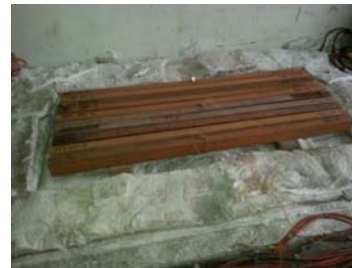
Figure 2. The samples arrangement in the heat treatment electrical furnace
