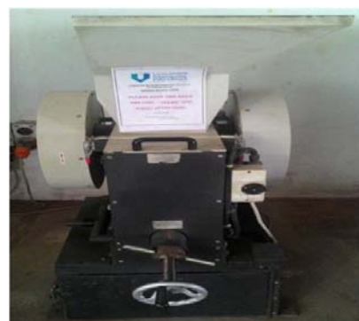
Figure 2. Jaw crusher used to produce fine sand.
