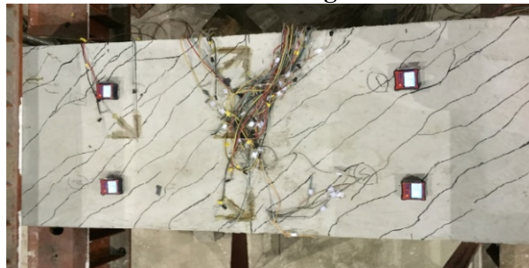
Figure 16. The cracks on the top face of SP1.
