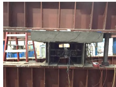
Figure 15. The cracks on the end face of SP1.
