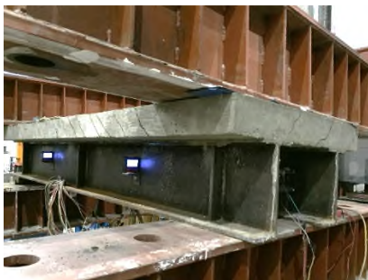
Figure 14. The cracks on the side face of SP1.
