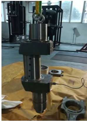
Figure 1. Free suspension diagram of crankshaft.
