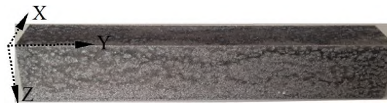
Figure 2. The specimen fabricated by the SLM.
