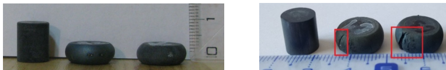
Figure 3. Specimens after the THT and compression test of a) Ti6Al4V and b) Ti26Nb (cracking in red boxes).
