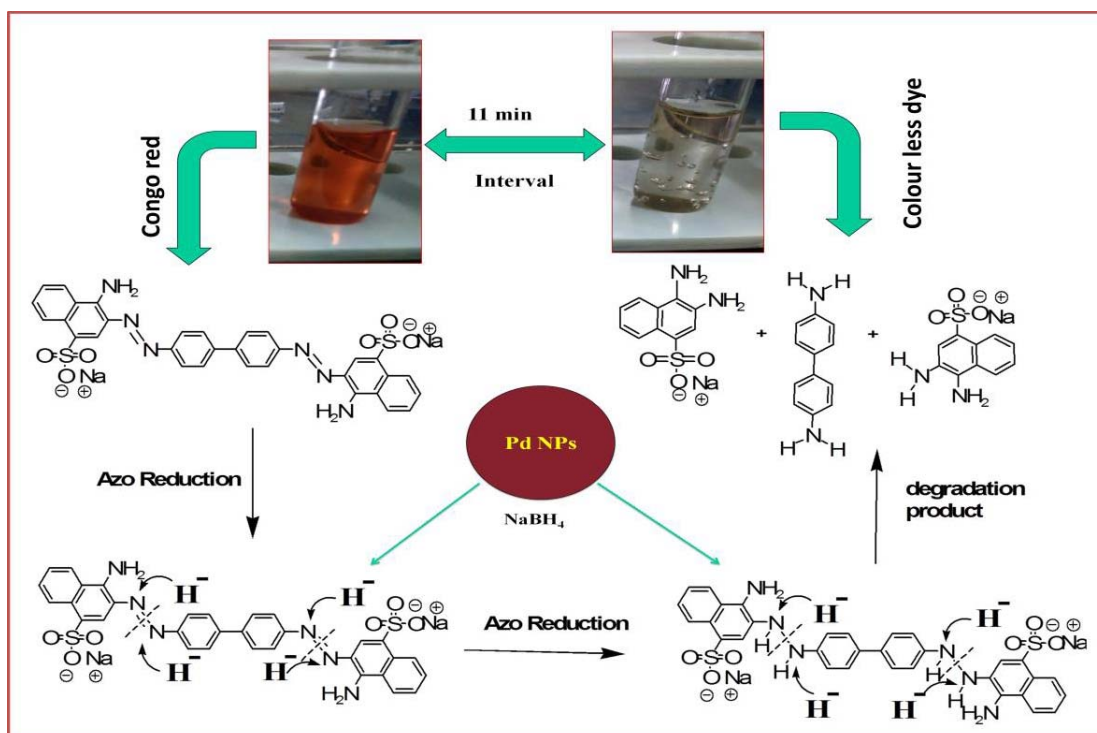
Fig. 8 The possible mechanism of Congo red dye degradation in the presence of NaBH 4 .
