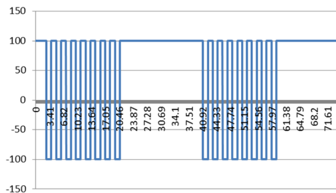
Figure 7. Control Pulse for solenoid valve 4
