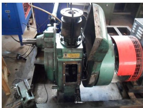
Figure 2. Photographic view of the dismantled engine before endurance test
