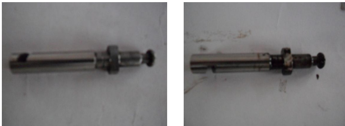
Figure 7. Deposits and wear traces on the plunger after the endurance test
