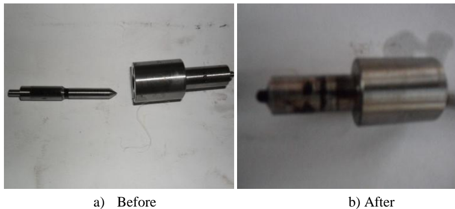
Figure 5. Comparison of nozzle and needle earlier and after the endurance test
