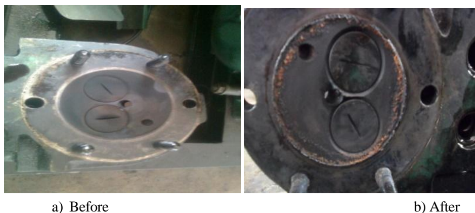
Figure 3. Comparison of cylinder head deposits earlier and after the endurance test
