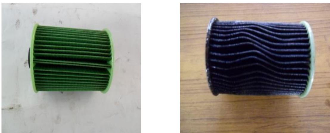
Figure 8. Comparison of fuel filter earlier and after the endurance test
