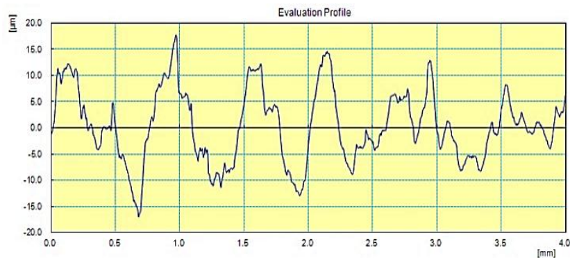
(a) Roughness profile of ASS 316L ( R_a = 5.584\mu\text{m} )
