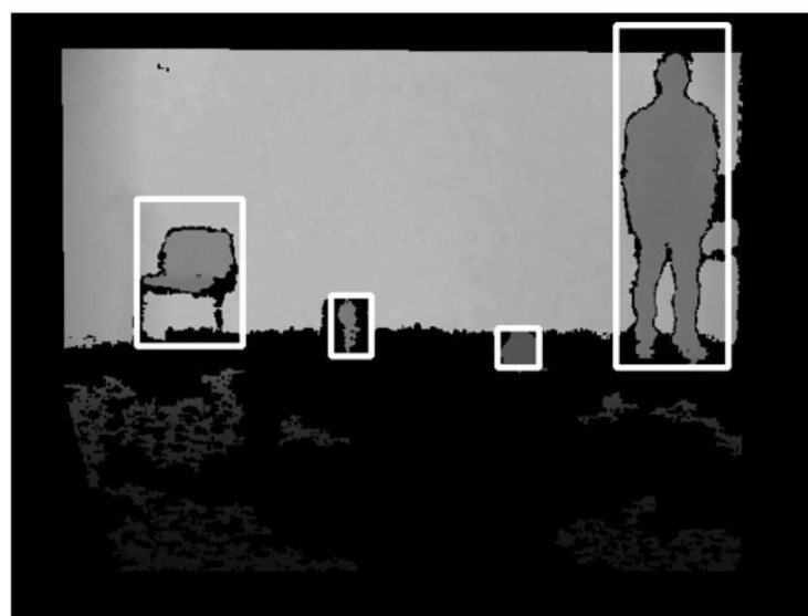
Figure 4. The depth image, which is enhanced by the detection results of YOLOv2. The bounding boxes select the interesting areas for the Object Locator.
