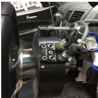
Figure 2. Steering Angle and torque sensors.
