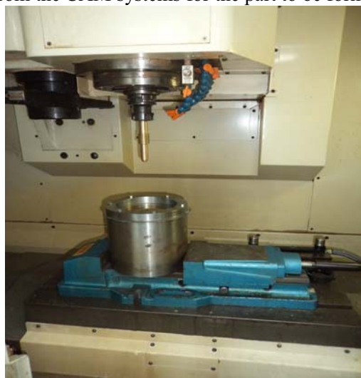
Figure 1. Setup of ISF process on the CNC milling machine table [17].
