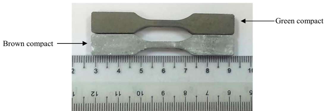
Figure 4. Green and brown compact of CoCrMo Alloy without defects.
