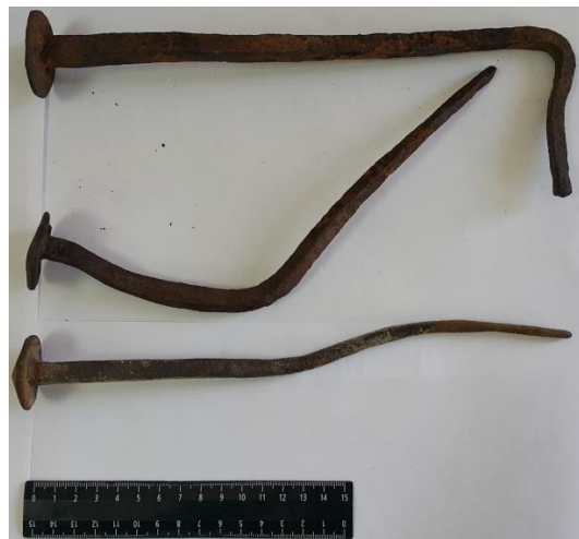
Figure 3. Three nails taken from the first wreck as specimens for metallurgical analysis. Top – Type B; bottom (2) – Type A. All specimens were bent. The first nail was bent deliberately for additional structural strength; the second specimen demonstrates deformation caused by torque (apparently the wooden member was twisted around the axis of the nail)
