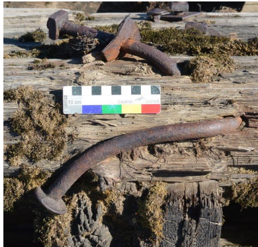
Figure 4. Two bolts, square washer, and square nut with scale marker. These two samples were bent
