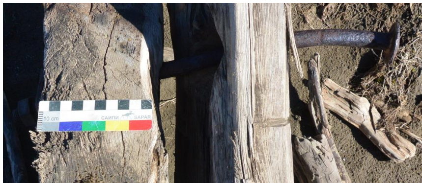
Figure 5. Demonstrates the length of the bolt holding two wooden members of the ship frame. The bolt and the wooden members are deformed due to shear stress
