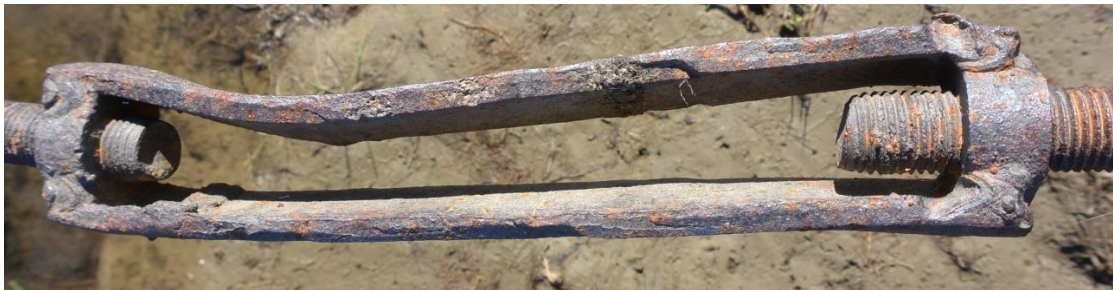
Figure 6. A turnbuckle with two threaded rods from wreck A. The weld is clearly seen. The upper plate buckled
