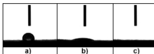
Figure 7. Dynamic contact angles of water drop on a) untreated PET; b) PET treated with PEG (1000) and DMDHEU (60 g/L); c) PET treated with PEG (2000) and DMDHEU (60 g/L).
