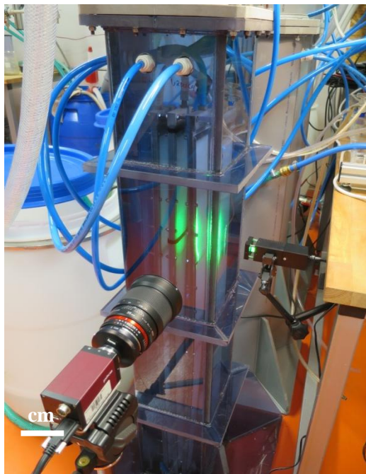
Figure 2. Picture of the filtration chamber from plexiglass and the visualization system.
