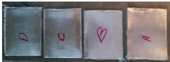
Figure 2. The used composite samples for impact resistance test
