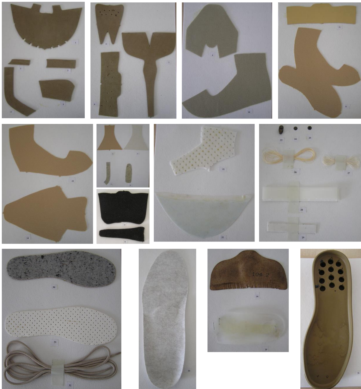
Figure 4. Structural parts of multifunctional boots for hot environment condition.
