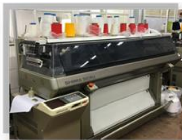
Figure 2. 10 gauge-flat bed knitting machine
