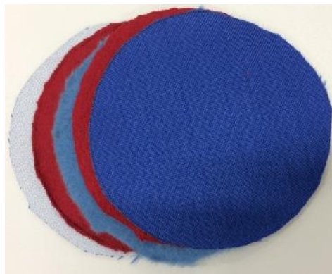
Figure 7. Five layered sandwich structure with highest thermal comfort (S5)
