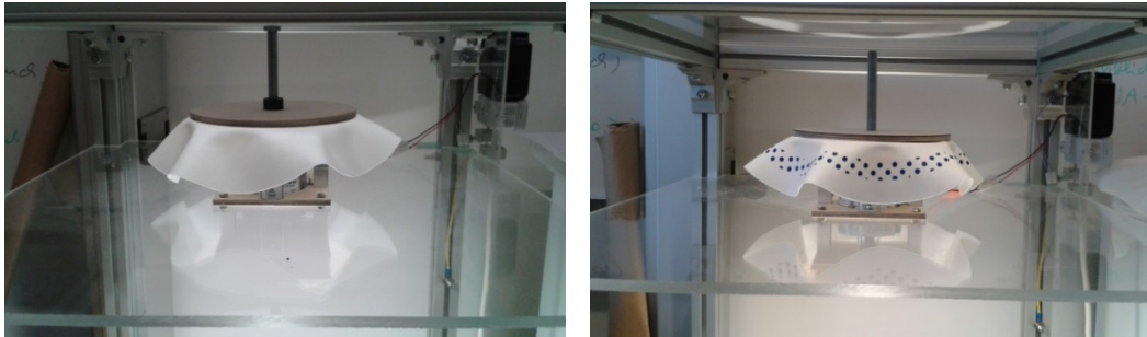
Figure 2 Drape test of pure textile fabric (left) and a fabric with a 3D-imprinted pattern (right panel).
