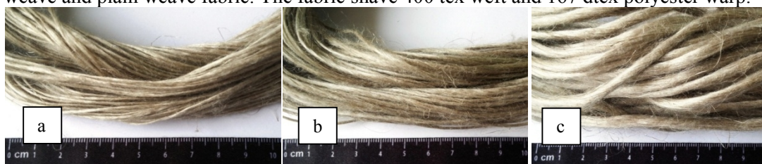
Figure 2. Flax roving plain a) 200 tex, b) 400tex, c) 2000tex
