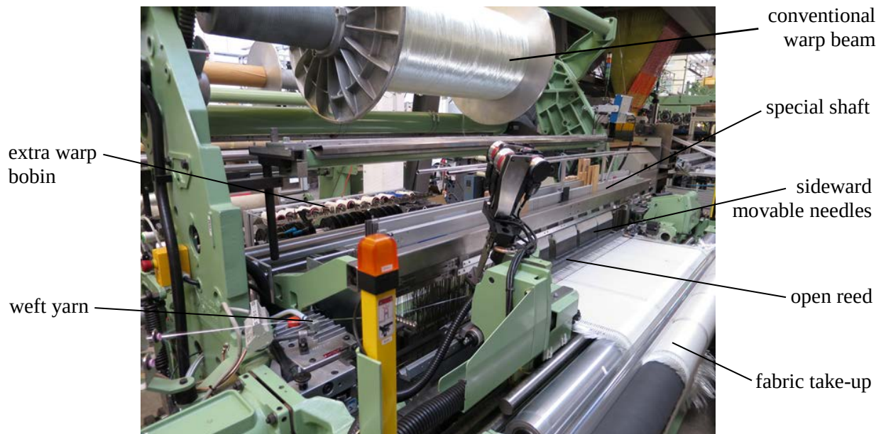
Figure 2. Rapier weaving machine with ORW function PTS 4/SOD.
