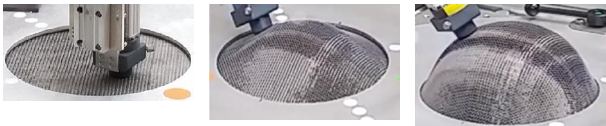
Figure 3. Scanning process for punch heights h = 0 mm, h = 50 mm and h = 100 mm (left to right).
