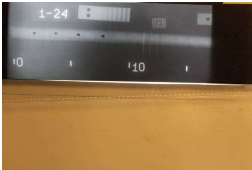
Figure 1a X-ray of object joint № 1-20. Defect of weld joint as a result of procedure violation (rapid water cooling); desired signal 14 dB. Crack under weld.
