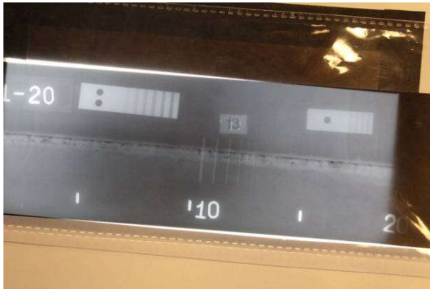
Figure 1b X-ray of weld joint №1-24. Hollow aperture under weld. Desired signal 12dB.
