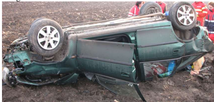
Figure 2 – the vehicle's front and rear part deformations
