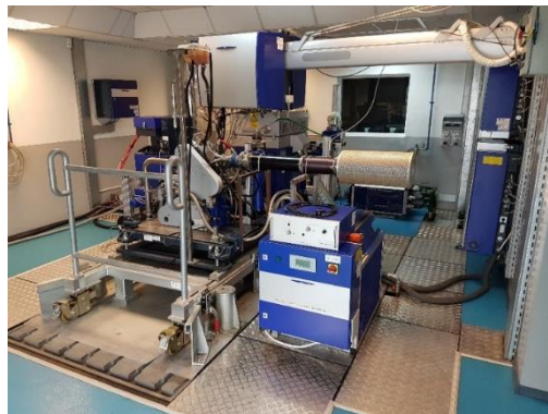
Figure 1. TESTECOCEL Laboratory set-up for SCRE AVL 5402
