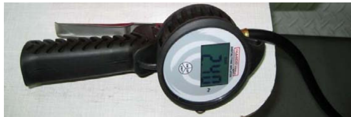
Figure 5. Measurement of tyre inflation pressure using a pressure gauge with digital display
