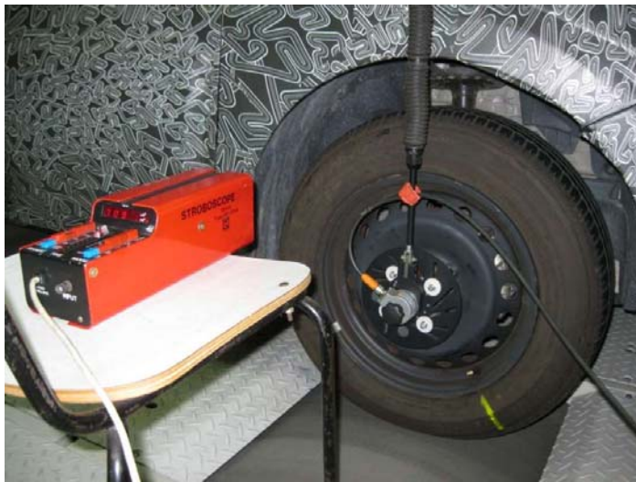
Figure 3. Measurement of wheel angular velocity using the stroboscopic lamp and the rotary encoder
