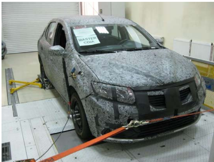
Figure 1. Passenger car used for experimental research on the chassis dynamometer
