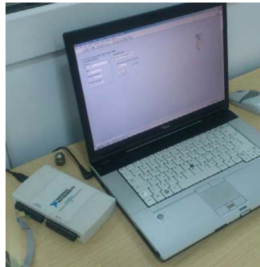
Figure 4. Data acquisition system for measuring wheel angular velocity
