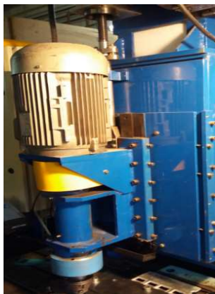
Figure 7. Force traducer type AM fixed on the welding machine
