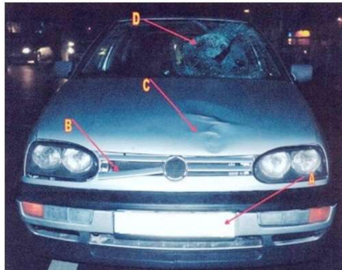
Figure 5. The damage caused to the VW vehicle after the impact with pedestrian
