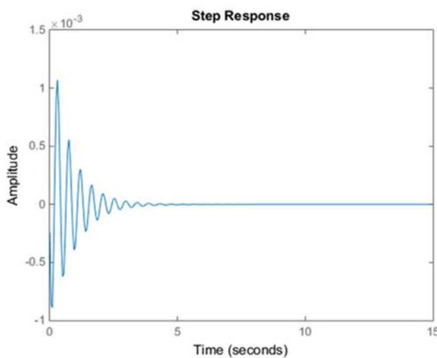
**Figure 8.** Closed-Loop Response with PID Controller for  $c_1 = 1000 \text{ [N*s/m]}$
