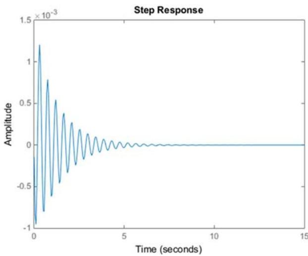
**Figure 7.** Closed-Loop Response with PID Controller for  $c_1 = 600 \text{ [N*s/m]}$
