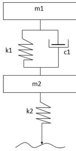
**Figure 4.** Suspension passive.
