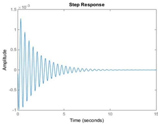
**Figure 6.** Closed-Loop Response with PID Controller for  $c_1 = 400 \text{ [N*s/m]}$
