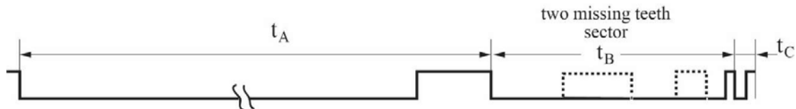
Fig.9 Time evolution for pulses coming from a crank wheel with 60-2 teeth configuration which is accelerated from 50 rpm to 5000 rpm in a very brief time
