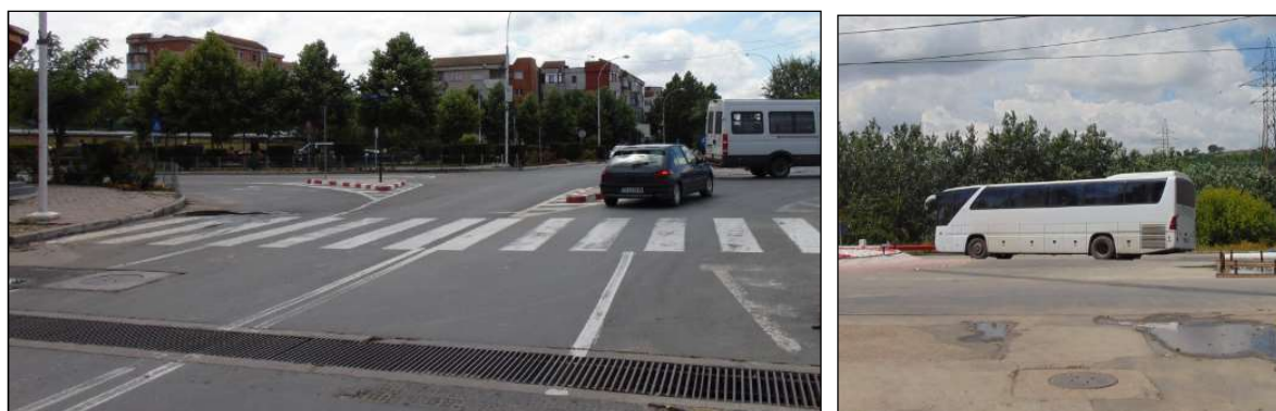
Figure 7. High noise sources for Route 1 - metallic drainage channels on the main road (left) and traffic composition: commuting buses (right)
